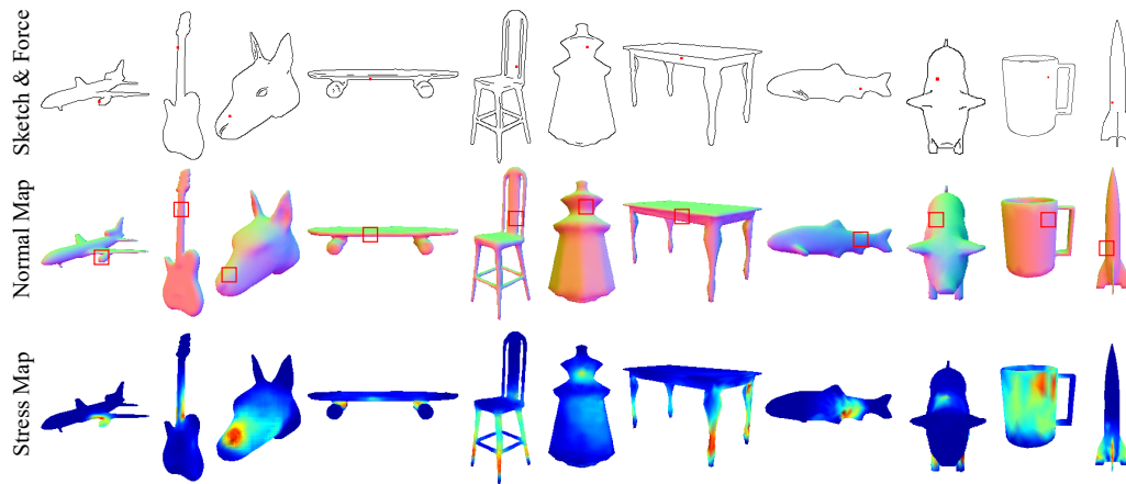
Fig. 4.6. Result gallery of eleven categories in our synthetic sketch-to-stress dataset. The top row shows the input sketches and external force locations (plotted as red dots), while the middle and bottom rows are our generated normal maps (with predicted force directions at the center of red boxes) and synthesized stress maps, respectively. Please zoom in to examine the details of the applied force locations/directions and the generated structural stress results.
